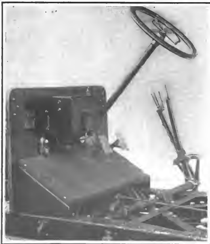
The Dash Carries the Six-Unit Coil and the Oiler Tell-Tale
